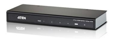
The VS184A HDMI Splitter is the perfect solution for anyone who needs to send one source of digital high definition video to four displays at the same time. It supports all HDMI-enabled equipment, such as DVD players, satellite set-top boxes and all HDMI displays.
