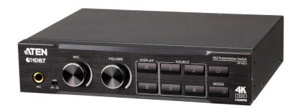
The ATEN VP1421 is a multi-in-one <u>presentation switch</u> that integrates a <u>video matrix</u> switch, 4K scaler, HDBaseT extender, audio DSP, and <u>analog</u>-to-digital converter functions into one compact device that easily mounts under a table or in a rack. With four <u>analog</u>/digital inputs to one HDBaseT and one HDMI\_<u>True 4K</u> outputs, it is designed to boost the efficiency and impact of professional <u>presentations</u>.
