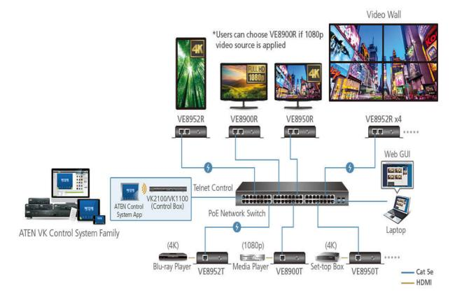
\*Note: VE8952 supports PoE and can be installed in combination with PoE network switches to reduce power cabling and additional power outlets. Before choosing the Network switch and installation, please refer to the Implementation Guide.
