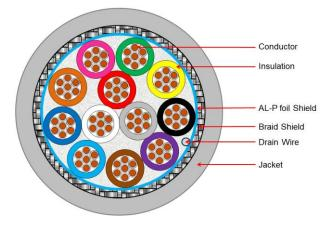
LINK Multi-Core cable,12 cores Double Shield
