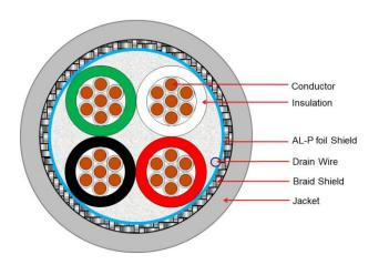
LINK Multi-Core cable, 4 cores Double Shield
